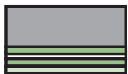
EC-1250N - semi-closed EPDM foam (EC-1200N) - Acrylic-based adhesive - Non-woven carrier - Acrylic-based adhesive - Release liner
