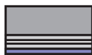
686CEP - Soft-closed cell foam - Acylic-based adhesive - Non-woven carrier - Acylic-based adhesive - Release liner
