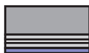
686C - Soft-closed cell foam - Acylic-based adhesive - Non-woven carrier - Acylic-based adhesive - Release liner
