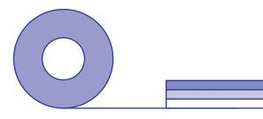
\* 733TOW has the same construction as 733T, but is winded with the release liner on the inside of the roll.
